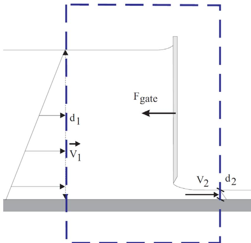
**2:** The application of the *continuity principle* gives the flow velocity upstream and downstream of the gate.
