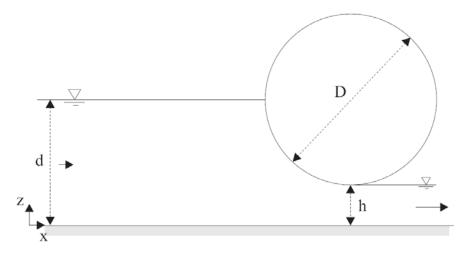
Solution (Drum gate) (a) d = 3.0 m (b) F = 340 kN
