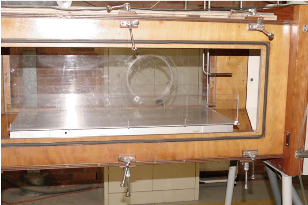
Fig. 2-2 - Photograph of the boundary layer experiment: smooth plate - Wind flow from right to left
