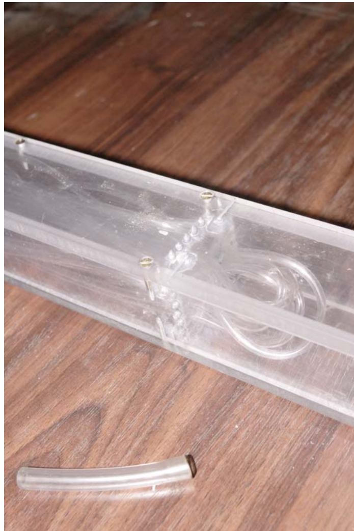
Fig. I-3 - Building model - Details of the pressure tapings
