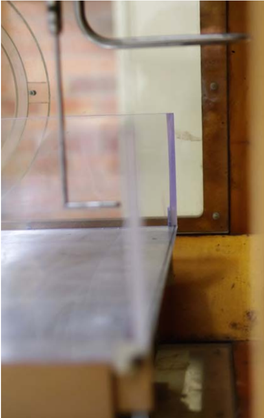
Fig. III-6- Wind tunnel boundary layer plate - Details of the plate leading edge and trip wire - Wind flow direction from right to left
