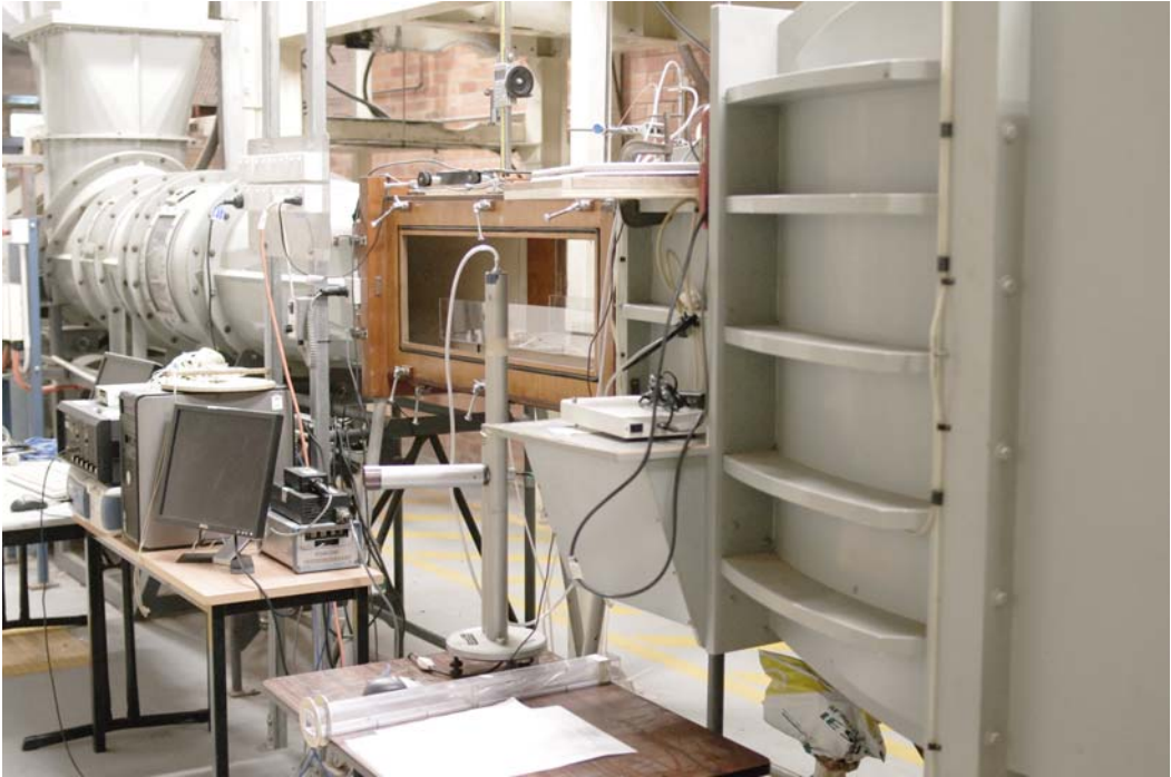
Fig. III-3 - Wind tunnel test section - Wind flow direction from right to left
