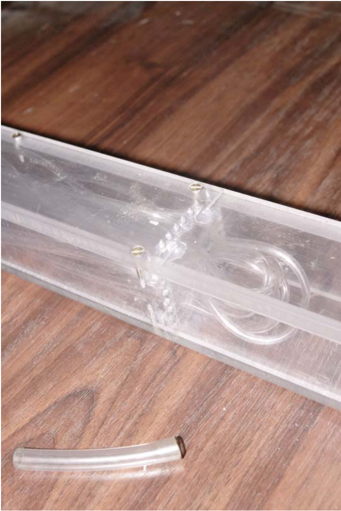
Fig. I-3 - Building model - Details of the pressure tapings
