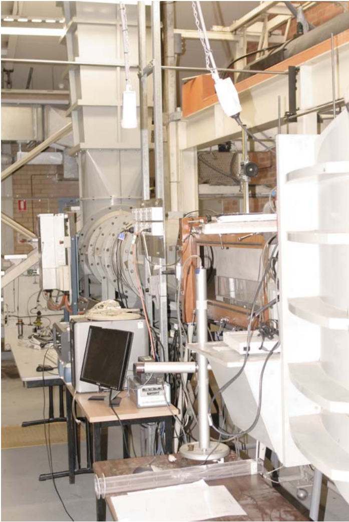
Fig. III-3 - Wind tunnel test section - Wind flow direction from right to left
