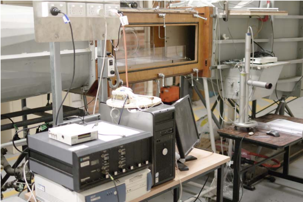
Fig. III-5 - Wind tunnel test section and boundary layer plate - Wind flow direction from right to left
