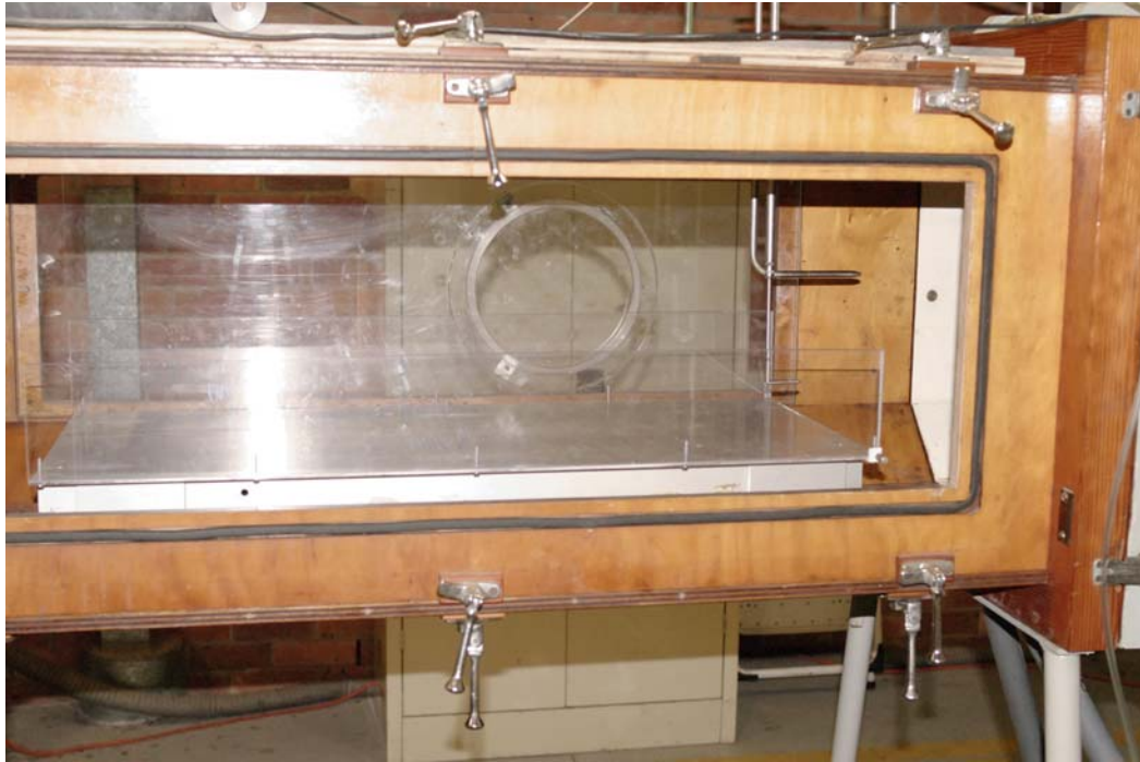
Fig. 2-2 - Photograph of the boundary layer experiment: smooth plate - Wind flow from right to left, with the Pitot tube on the right of the photograph
