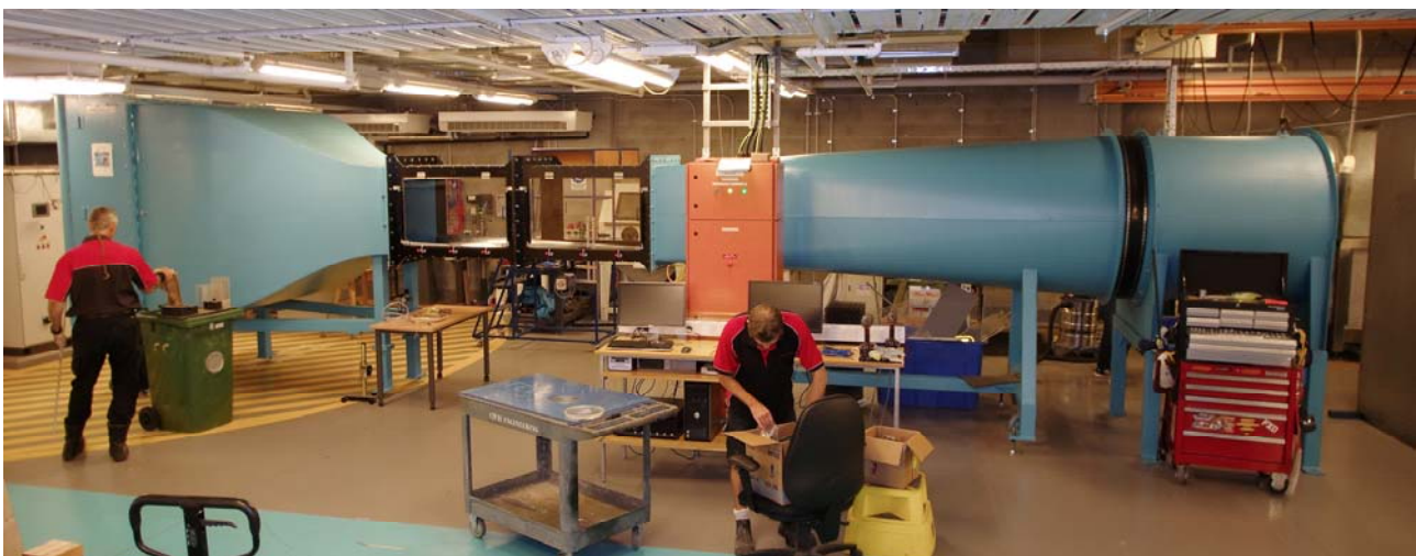
Fig. 2-1 - Photographs of wind tunnel experiment (A) Sideview with flow direction from left to right
