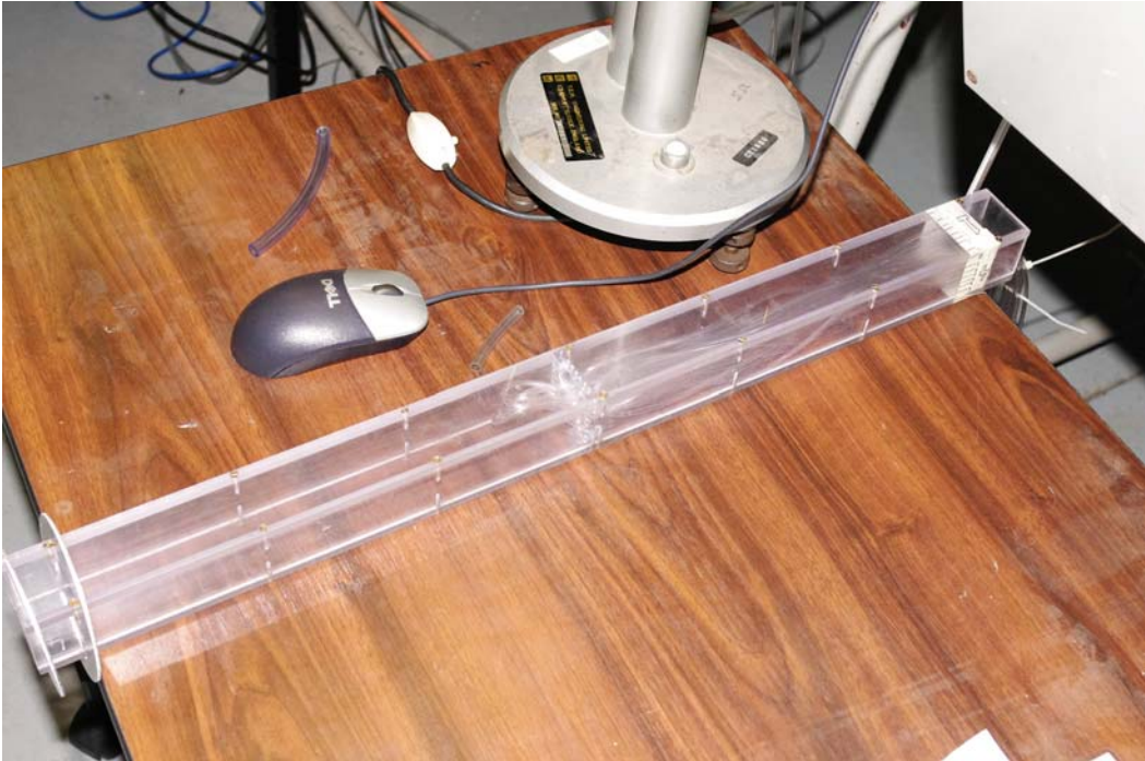
Fig. I-2 - Building model - Inside details of the pressure tappings
