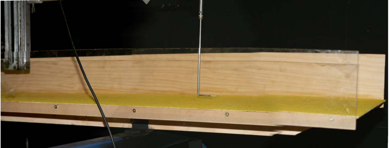
Fig. 2-2 - Photograph of the boundary layer experiment: rough plate (sand paper grade 40) - The hot-wire probe is located at x = +0.30 m and y = 0.010 m - Wind flow from right to left
