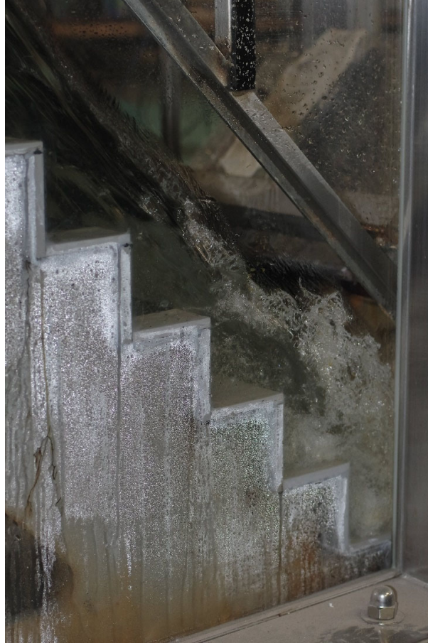
Fig. A-1 - Experimental channel with flat horizontal steps ( h = 0.1 m) - Flow conditions: d_c/h = 1.6 , Re = 8.0 \times 10^5 - View through the right sidewall
