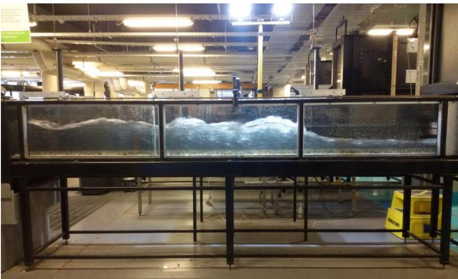
**Figure 1.** Initial setup of flume for recording videos with high speed cameras; up: LED light and wall for smooth bed condition and down: LED for rough bed, flow condition:  $Q = 0.06218 \text{ m}^3/\text{s}$ ,  $d_1 = 0.082\text{m}$   $Fr_1 = 1.78$ ,  $x_1 = 1\text{m}$  and flow from right to left.
