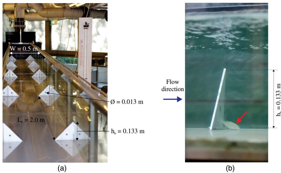
**Fig. 1.** Experimental channel: (a) flume equipped with two rows of baffles (double-sided baffles,  $h_b = 0.133$  m;  $L_b = 2.0$  m; and  $\phi 13$ -mm hole) looking upstream; and (b) juvenile silver perch (*Bidyanus bidyanus*) resting downstream of a baffle (single-sided baffles,  $h_b = 0.133$  m;  $L_b = 0.67$  m; and  $\phi 13$ -mm hole), with flow direction from left to right ( $Q = 0.0556$  m<sup>3</sup>/s). Arrow points to the fish.
