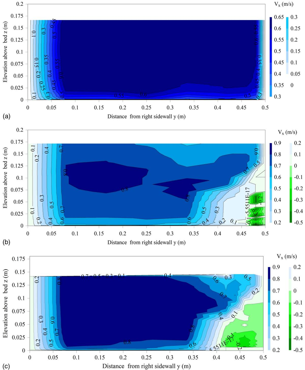
**Fig. 2.** Contour plots of local time-averaged velocity  $V_x$  (m/s) in smooth and corner baffled channels for  $Q = 0.0556$  m<sup>3</sup>/s: (a) smooth flume channel,  $x = 8.15$ ; and  $d = 0.171$  m; (b) plain baffles in left corner,  $d = 0.172$  m;  $h_b = 0.133$  m;  $L_b = 1.33$ ;  $x_b = 8.12$  m; and  $x - x_b = 0.03$  m; and (c) baffles with hole in left corner,  $d = 0.172$  m;  $h_b = 0.133$  m;  $L_b = 0.67$  m;  $\phi = 13$  mm hole;  $x_b = 8.12$  m; and  $x - x_b = 0.03$  m.
