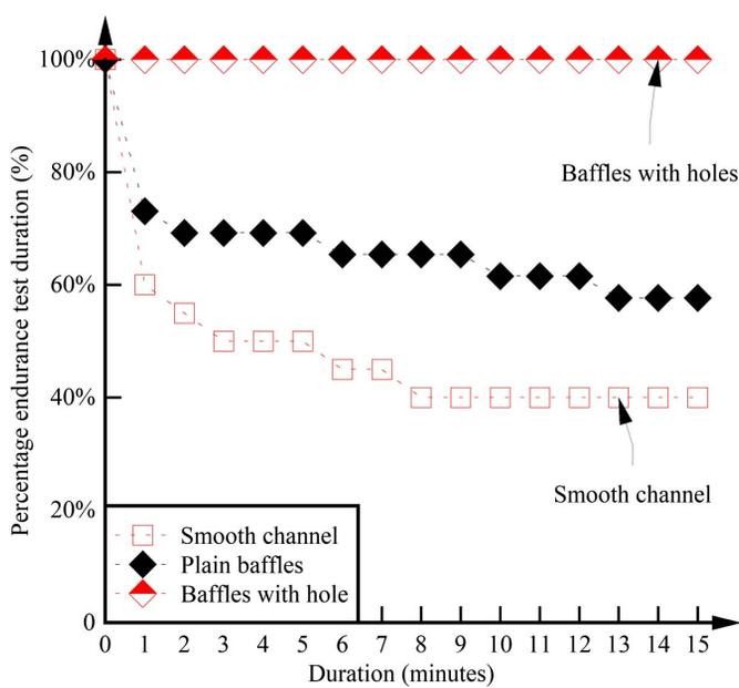
**Fig. 4.** Cumulative endurance test duration data for juvenile silver perch (*Bidyanus bidyanus*) negotiating upstream passage in the 12 m in length and 0.5 m in width culvert barrel flume:  $Q = 0.0556 \text{ m}^3/\text{s}$ ;  $S_o = 0$ ; test duration: 15 min. Comparison between all three boundary configurations (Table 2). Baffle characteristics:  $h_b = 0.133 \text{ m}$ ; and  $L_b = 0.67 \text{ m}$ .
