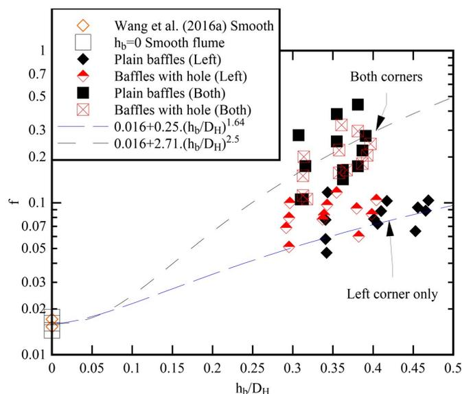
**Fig. 3.** Flow resistance in small corner baffle channel flows: Darcy-Weisbach friction factor as a function of the relative baffle height  $h_b/D_H$ , with baffles located in the left corner only and along both corners. Comparison with the smooth flume data of Wang et al. (2016a).
