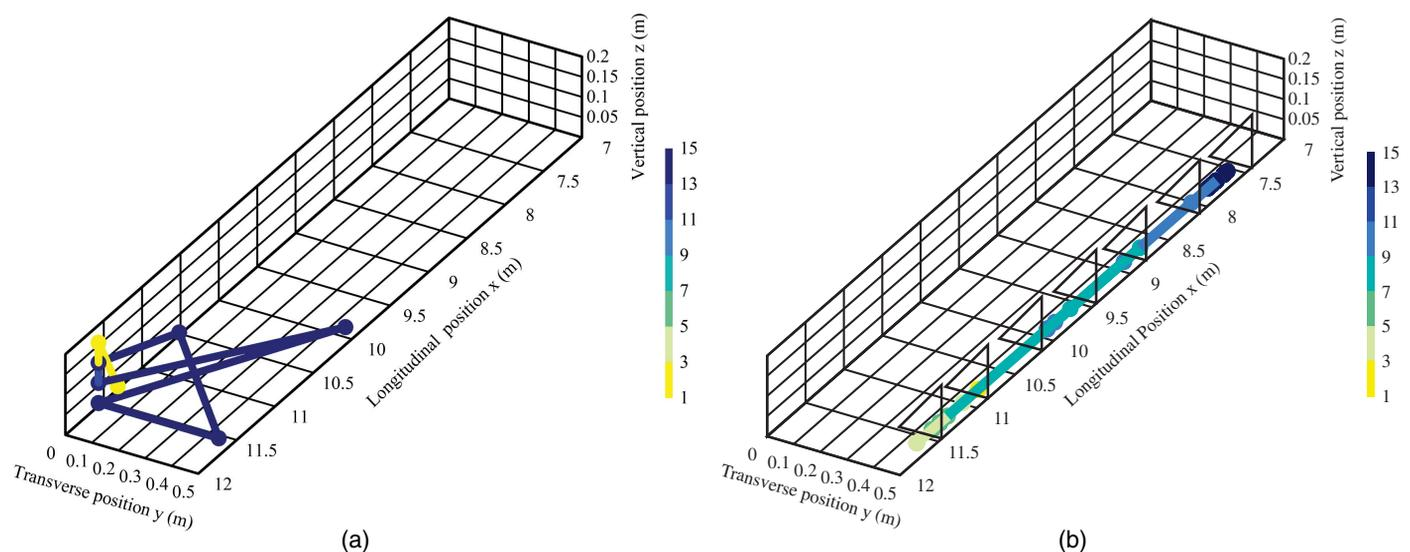
**Fig. 5.** Typical fish trajectories during fish testing:  $Q = 0.0556 \text{ m}^3/\text{s}$ ;  $S_o = 0$ ;  $W = 0.5 \text{ m}$ ; flow direction of top right to bottom left. Fish species: juvenile silver perch (*Bidyanus bidyanus*). The scale in minutes corresponds to test duration: (a) smooth flume; and (b) plain baffles:  $h_b = 0.133 \text{ m}$ ; and  $L_b = 0.67 \text{ m}$ . Baffles located along the left corner ( $y = 0.5 \text{ m}$ ).
