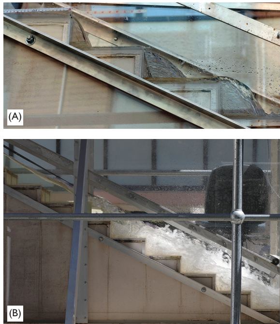
Figure 3.2 Nappe and skimming flows down a 1V:2H flat stepped chute ( h = 0.10 m). (A) Nappe flow, d_c/h = 0.13 . (B) Skimming flow, d_c/h = 1.45 .
