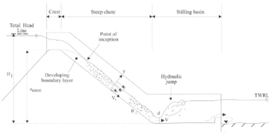
**Fig. 3.** Cross-sectional sketch of small dam spillway.
