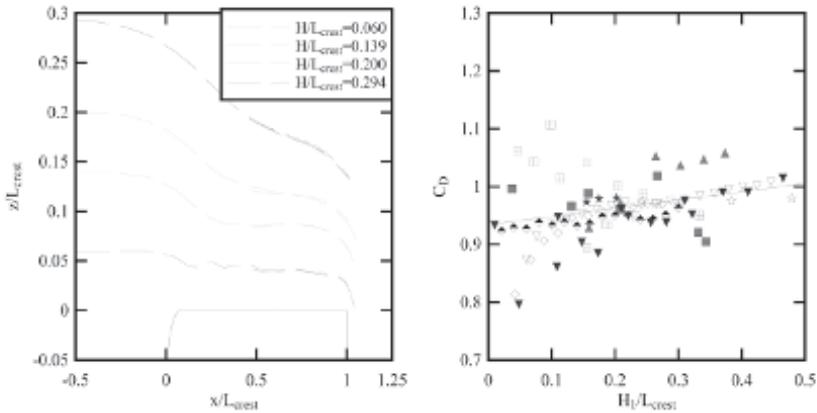
(A) Broad crested weir with upstream rounded corner: dimensionless free-surface profiles (Data: Felder and Chanson 2012) and dimensionless discharge coefficient data (Data: Vierhout 1973; Bazin 1896; Gonzalez and Chanson 2007; Felder and Chanson 2012; Zhang and Chanson 2015; Felder 2015).
