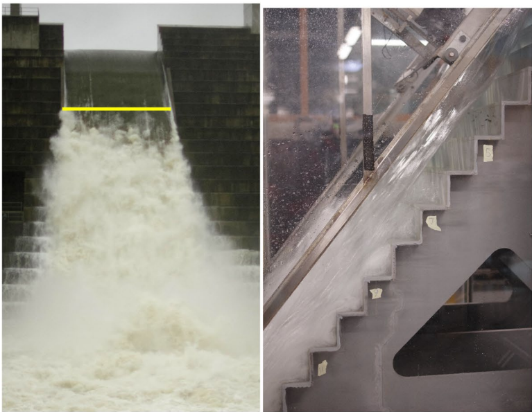
(B) d_w/h = 1.35 , Re = 4.0 \times 10^7 (Hinze Dam) and d_w/h = 1.33 , Re = 6.1 \times 10^5 (UQ model)
