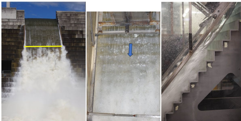
(C) d_w/h = 1.6 , Re = 5.1 \times 10^7 (Hinze Dam) and Re = 7.8 \times 10^5 (UQ model) - Centre: top view of laboratory chute flow (arrow show flow direction)
