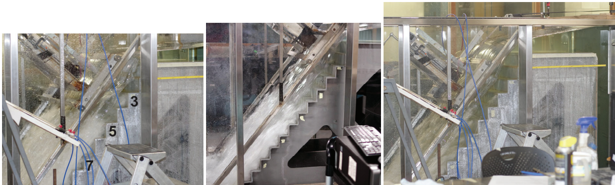
Figure 3. Laboratory experiments at the University of Queensland, h = 0.10 m, 1V:0.8H slope - From left to right: d_c/h = 0.98 , 1.33 and 1.58 - Step edge numbering shown in the left photograph.
