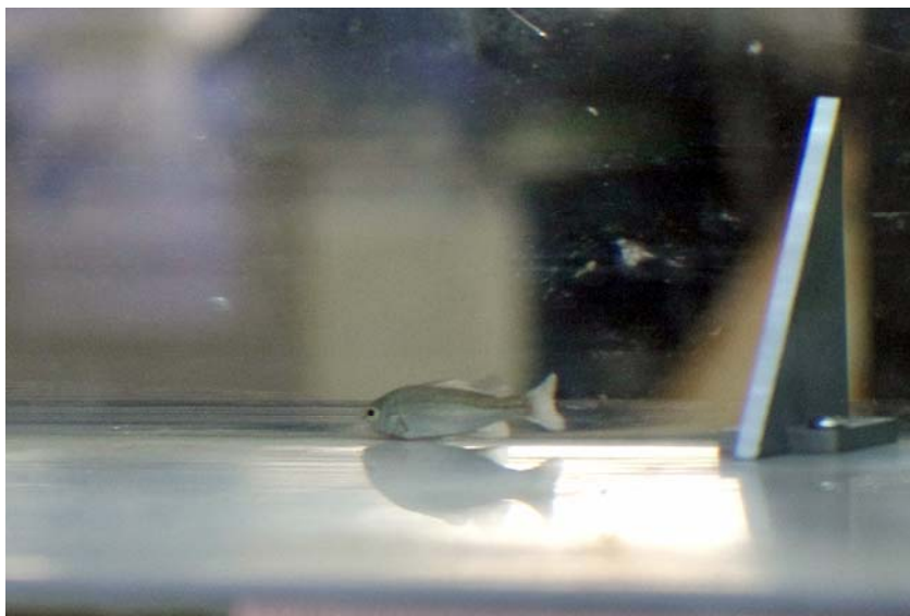
Figure 7. Juvenile silver perch ( Bidyanus bidyanus ) ( L_f = 49 mm, m_f = 1.4 g) swimming upstream in the bottom left corner of a 12 m long 0.5 m wide culvert barrel channel equipped with small triangular baffles on one side (Spacing L_b = 0.67 m, Height h_b = 0.067 m) against a steady flow ( Q = 0.0556 m 3 /s, V_{\text{mean}} = 0.684 m/s, d = 0.163 m, S_o = 0 ) - Flow direction from left to right, with fish resting upstream of a corner baffle about 9 m upstream of the outlet.
