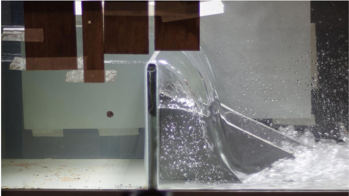
**Figure 3. Circular-crested weir overflow for  $Q = 0.01705 \text{ m}^3/\text{s}$  and  $d_1 = 0.321 \text{ m}$  (with detached nappe). Flow direction from left to right.**
