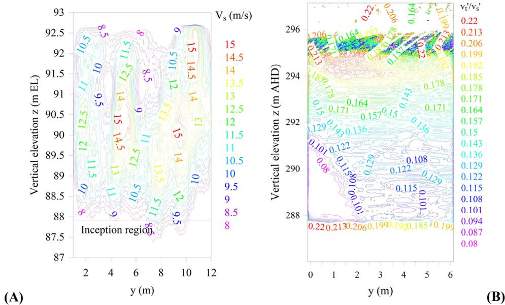
**Figure 4. Optical velocity measurements at prototype spillways. (A) Contour map to time-averaged-surface velocity  $V_s$  in the on-aerated developing flow region at Hinze Dam Stage 3 on 24 March 2021 ( $Q = 140 \text{ m}^3/\text{s}$ ). (B) Contour map of the ratio  $v_t'/v_s'$  at Chinchilla MEL weir on 15 December 2021 ( $Q = 144 \text{ m}^3/\text{s}$ ).**
