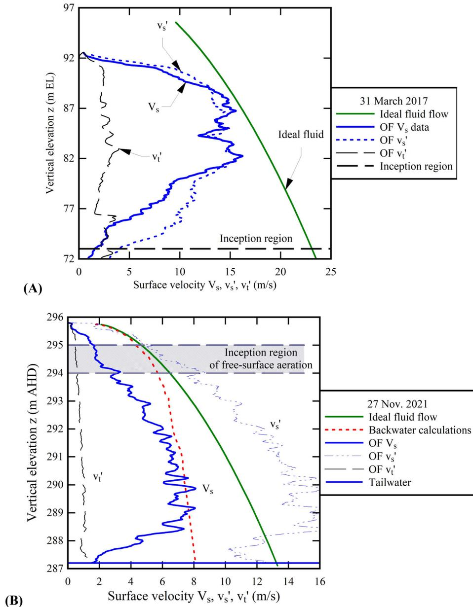
**Figure 2. OF surface velocity: comparison with theoretical estimates. (A) Comparison between optical flow (OF) surface velocity data and ideal fluid flow velocity at Hinze Dam Stage 3 on 31 March 2017 ( $Q = 334 \text{ m}^3/\text{s}$ ). (B) Comparison between optical flow (OF) surface velocity data and backwater calculations at Chinchilla MEL weir on 27 November 2022 ( $Q = 121 \text{ m}^3/\text{s}$ ).**
