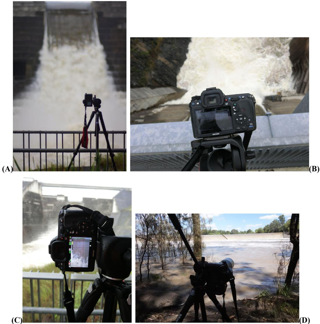
**Figure 3. Optical measurement setup at prototype spillways. (A) Hinze Dam Stage 3 on 4 March 2022 ( $Q = 111 \text{ m}^3/\text{s}$ ). (B) Hinze Dam Stage 3 on 4 March 2022 ( $Q = 111 \text{ m}^3/\text{s}$ ). (C) Hinze Dam Stage 3 on 3 March 2022 ( $Q = 143 \text{ m}^3/\text{s}$ ). (D) Chinchilla MEL weir on 27 November 2022 ( $Q = 121 \text{ m}^3/\text{s}$ ).**
