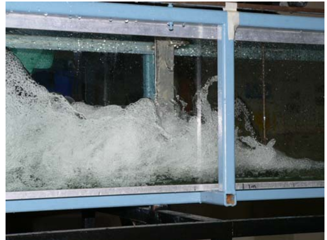
(A) Fr_1 = 6.7 , Re_1 = 9.4 \text{ E}+4 , x_1 = 1 \text{ m} , W = 0.25 \text{ m}
