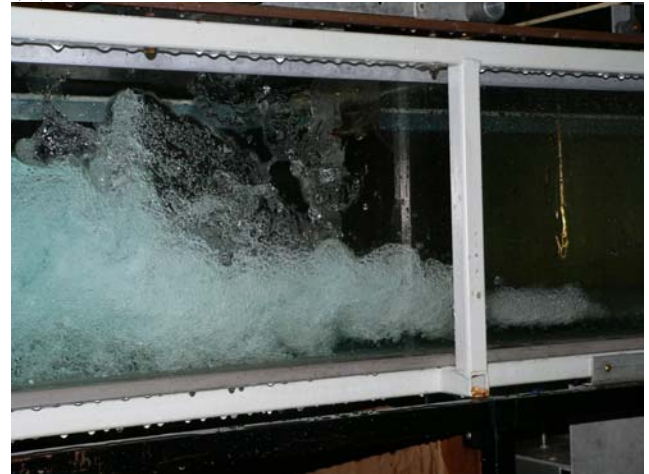
(B) Fr_1 = 8.6 , Re_1 = 9.8 \text{ E}+4 , x_1 = 1 \text{ m} , W = 0.5 \text{ m}
