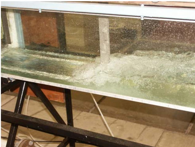
(A) Fr_1 = 5.1 , Re_1 = 2.4 E+4 , x_1 = 0.5 m, W = 0.25 m (shutter speed: 1/60 s)
