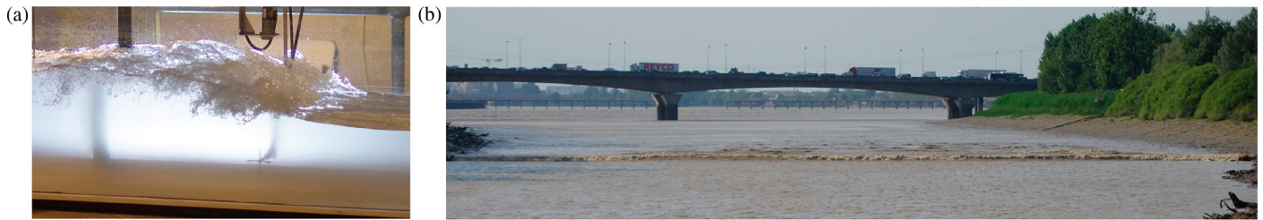
Figure D1 Breaking surge propagation: (a) laboratory study in a 19 m long 0.7 m wide flume – bore propagation (from left to right) against the initial flow direction; (b) field measurements in the Garonne River (France) – bore propagation background to foreground
