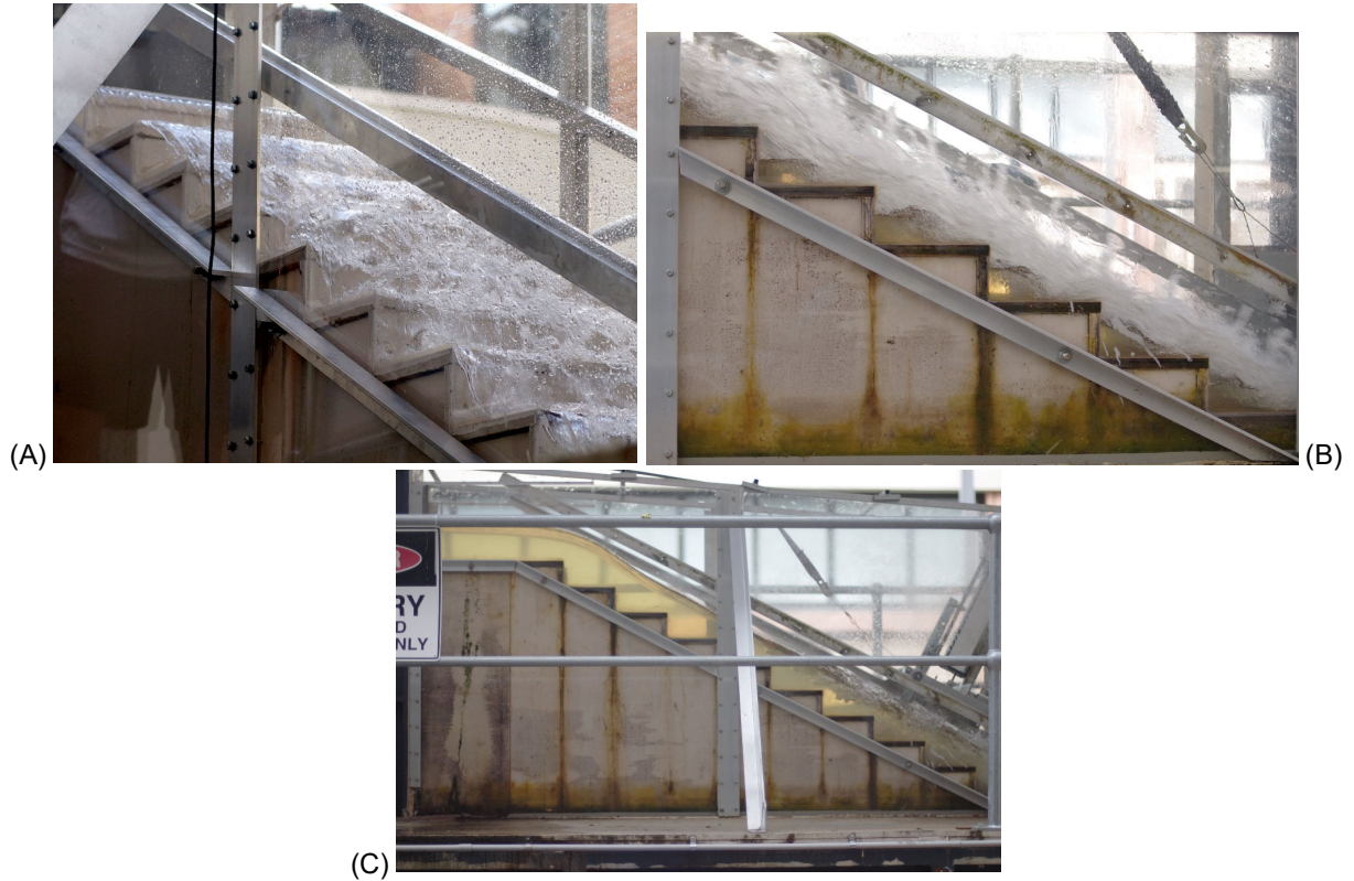
Figure 3. Flow regimes on a stepped spillway model: 1V:2H ( \theta = 26.6^\circ ), h = 0.10 m (University of Queensland). (A) Nappe flow ( d_c/h = 0.133 ); (B) Transition flow ( d_c/h = 0.8 ); (C) Skimming flow ( d_c/h = 1.5 )
