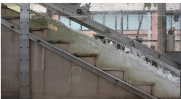
Figure 1. Air-water flows downstream of the inception point of free-surface aeration on a stepped spillway ( \theta = 26.6^\circ ); skimming flow regime; d_c/h = 1.25 , q_w = 0.137 \text{ m}^2/\text{s} , Re = 5.5 \times 10^5
