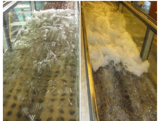
(A) Hydraulic jump with small roller and wavy free-surface: Fr_1 = 2.8 ; Q_w = 0.03 m 3 /s; Re = 6.0 \times 10^4 ; h = 0.058 m; Re = 1.2 \times 10^5 ; h = 20 mm (flow from top to bottom) (B) Jump with stable roller and wavy free-surface: Fr_1 = 4.3 ; Q_w = 2.8 m 3 /s; Re = 6.0 \times 10^4 ; h = 0.058 m; Re = 1.2 \times 10^5 ; h = 20 mm (flow from bottom to top)
