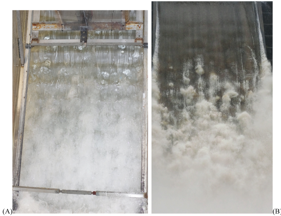
Fig. 5. Air-water skimming flow down 51.3° staircase chutes under Froude similar conditions ( h/d_c = 0.63 ), with flow direction from top to bottom - (A) Laboratory channel, Q = 0.193 \text{ m}^3/\text{s} , h = 0.1 \text{ m} , h/d_c = 0.63 , Re = 1.95 \times 10^5 , shutter speed: 1/100 \text{ s} ; (B) Hinze dam stepped spillway, Q = 143 \text{ m}^3/\text{s} , h = 1.5 \text{ m} , h/d_c = 0.63 , Re = 1.16 \times 10^7 , shutter speed: 1/640 \text{ s} .
