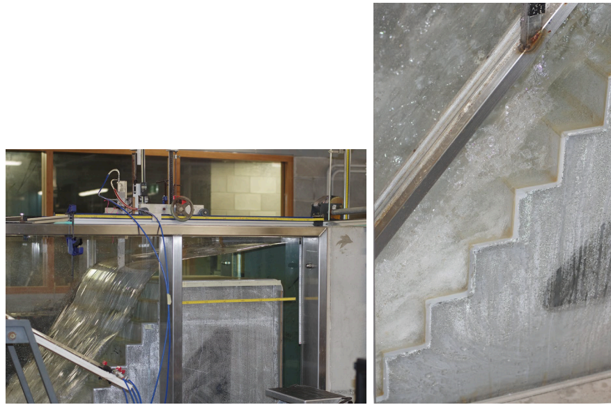
(A, Left) Flow above the broad-crest weir - Q = 0.150 \text{ m}^3/\text{s} , h/d_c = 0.75 , Re = 1.51 \times 10^5
