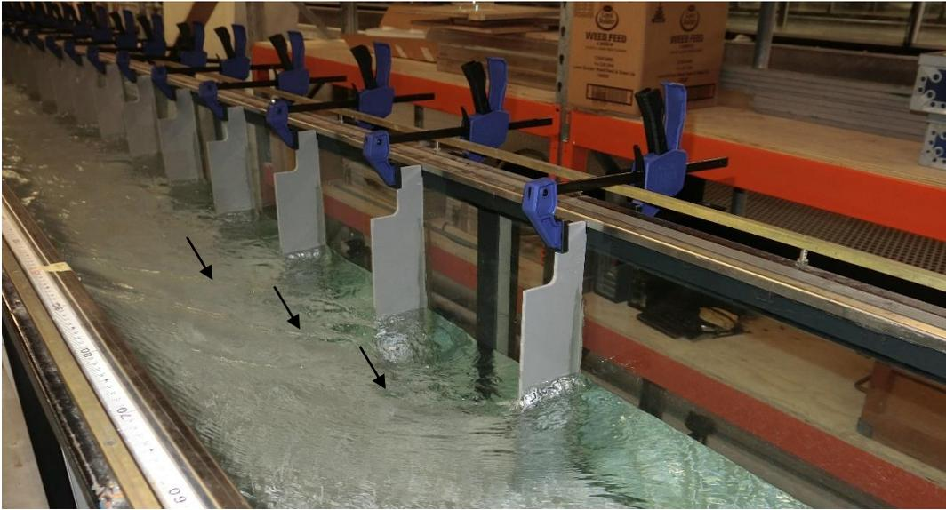
(a) Free-surface flow pattern in an open channel with medium side wall baffles  $h_b = 0.083$  m, distance between baffles  $L_b = 0.333$  m, flow rate  $Q = 0.056$  m<sup>3</sup>/s
