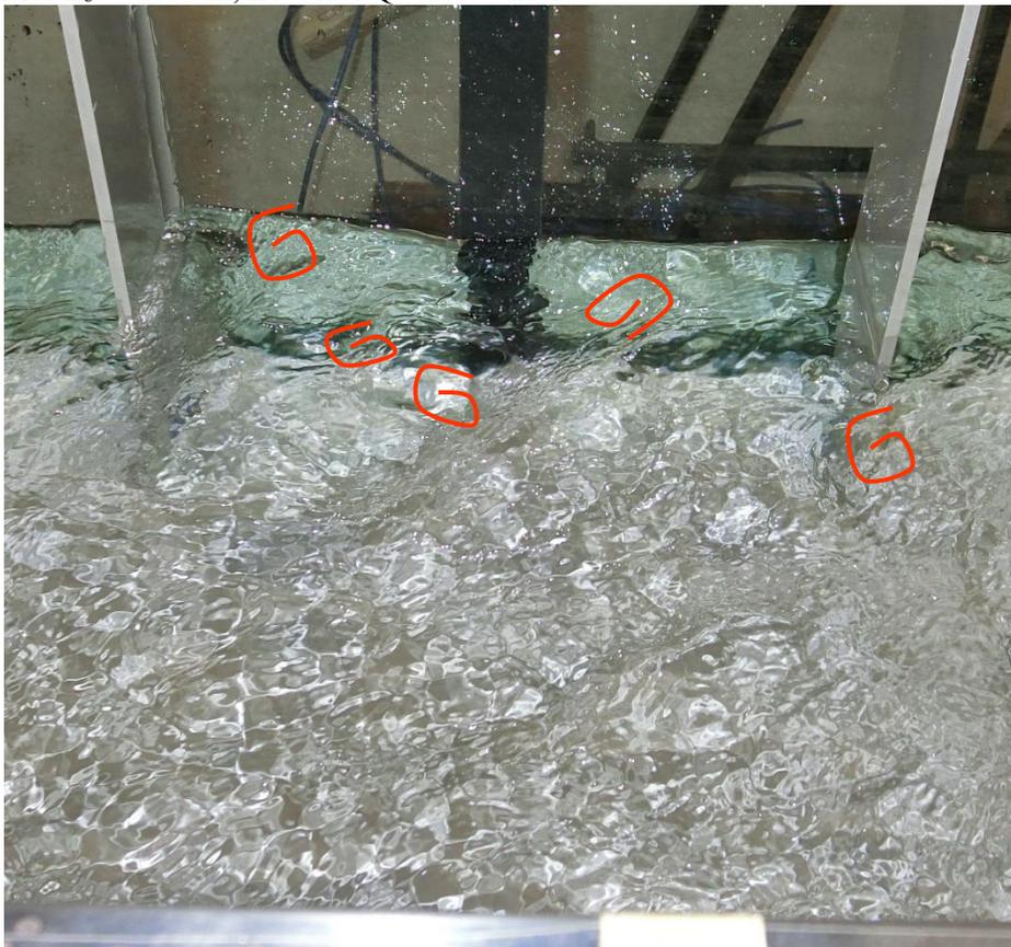
(b) Swirling flow structures observed in between two baffles ( $h_b = 0.083$  m,  $L_b = 0.333$  m,  $Q = 0.037$  m<sup>3</sup>/s)
