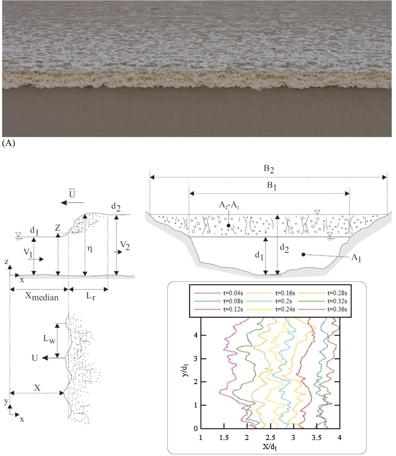
**Fig. 1.** Breaking tidal bore propagation. (A) Looking downstream at the Qiantang River bore in the northern channel downstream of Xinchang, China on 6 September 2013 at 11:50 –  $d_1 \sim 1$  m,  $\bar{U} \sim 3.6$  m/s,  $Fr_1 \sim 2.1$ . (B) Definition sketch – bottom left Inset: Instantaneous roller toe perimeter as function of time (Run 2)
