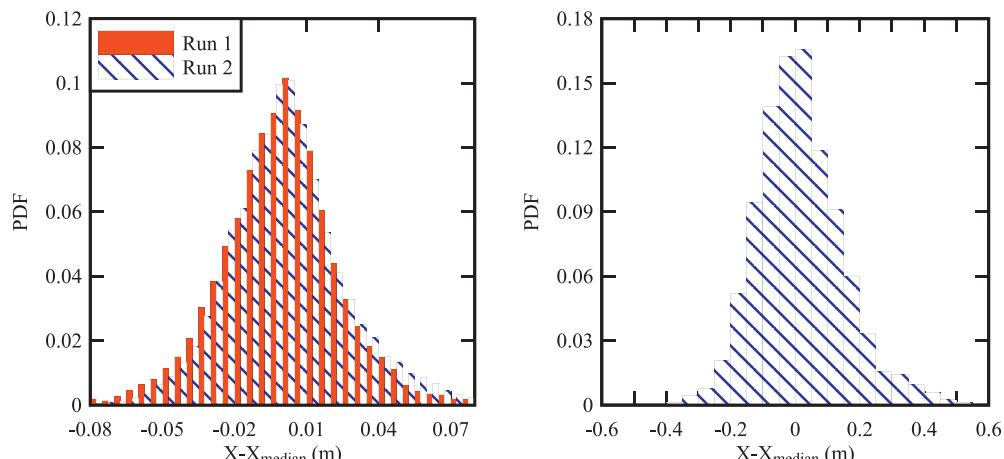
**Fig. 3.** Probability distribution function of longitudinal fluctuations in roller toe perimeter about the median – Left: laboratory data; Right: field data.
