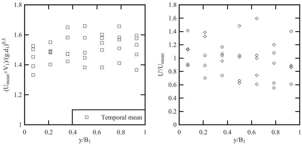
**Fig. 5.** Transverse variation in roller toe celerity and celerity fluctuations – Left: temporal mean celerity; Right: standard deviation.
