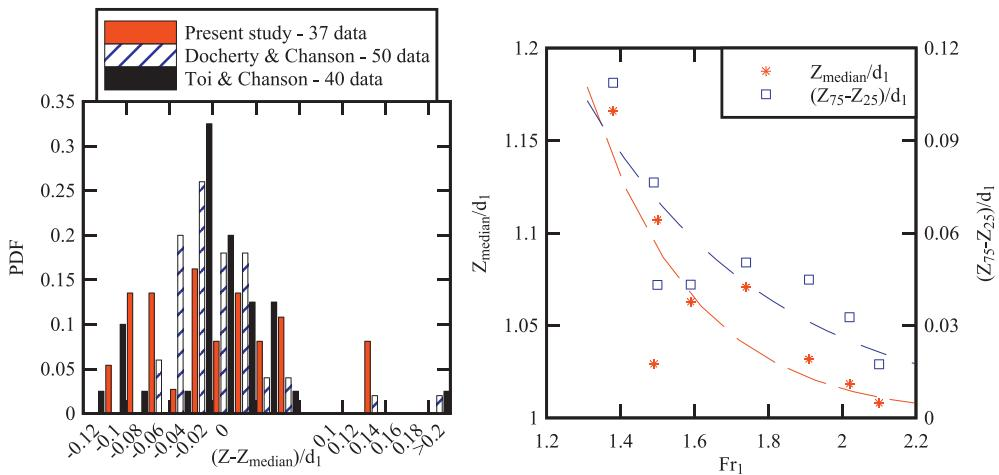
**Fig. 4.** Vertical elevation  $Z/d_1$  of roller toe – Left: probability distribution function of roller toe elevation about the median; Right: median elevation and difference between third and first quartiles – comparison between laboratory data.
