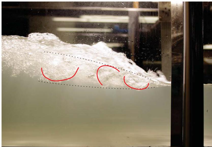
**Fig. 2.** Side view of coherent vortical structures in the shear layer of a roller –  $Fr_1 = 1.65$ ,  $Q = 0.085 \text{ m}^3/\text{s}$ , shutter speed: 1/125 s, bore propagation from left to right.
