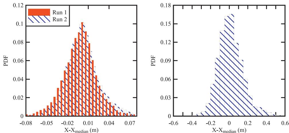
**Fig. 3.** Probability distribution function of longitudinal fluctuations in roller toe perimeter about the median – Left: laboratory data; Right: field data.
