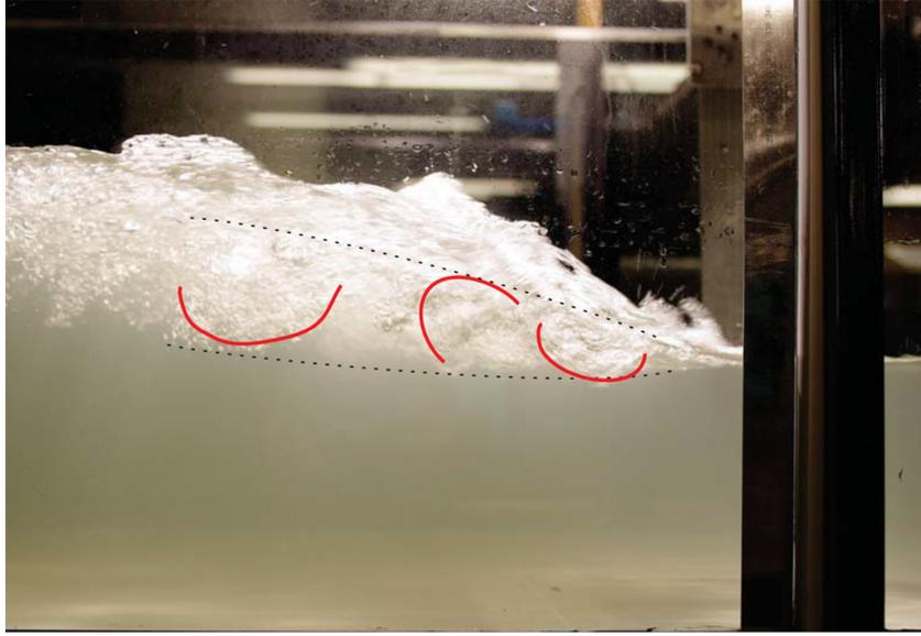
**Fig. 2.** Side view of coherent vortical structures in the shear layer of a roller –  $Fr_1 = 1.65$ ,  $Q = 0.085 \text{ m}^3/\text{s}$ , shutter speed:  $1/125 \text{ s}$ , bore propagation from left to right.
