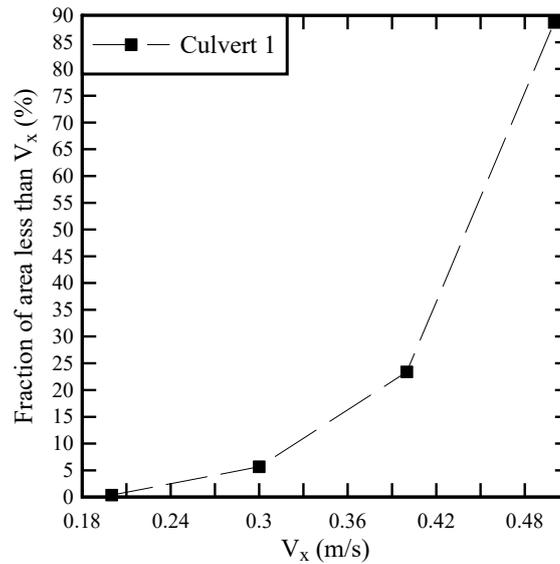
Fig. A-3 - Percentage of flow area under certain velocity values for a single cell in a seven-cell structure of case 1 (Culvert 1) at 10% of design flow ( $0.1 \times Q_{des} = 2 \text{ m}^3/\text{s}$ ); results near the downstream end of the culvert barrel (0.5 m upstream from the barrel exit)
