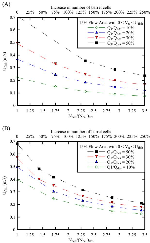
**Fig. 3** Relative increase in number of cells  $N_{cell}/(N_{cell})_{des}$  for fish-friendly multi-cell box culverts as a function of the threshold discharge  $Q_1/Q_{des}$  and characteristic fish swimming speed  $U_{fish}$ , with 15% of flow area where  $0 < V_x < U_{fish}$ . **a** Culvert 1, **b** Culvert 2
