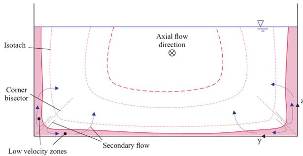
**Fig. 6** Sketch of low-velocity zones as defined by Eq. (1) in a box culvert barrel, looking downstream
