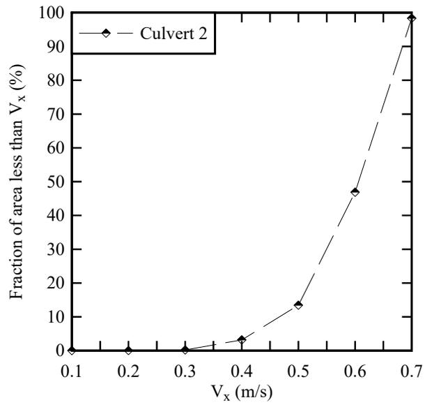
Fig. A-5 - Percentage of flow area under certain velocity values for a single cell in a six-cell structure of case 2 (Culvert 2) at 10% of design flow ( $0.1 \times Q_{des} = 0.48 \text{ m}^3/\text{s}$ ); results near the downstream end of the culvert barrel (2 m upstream from the barrel exit)
