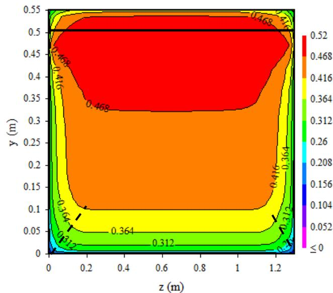
Fig. A-2 - Longitudinal velocity contour of a single cell in a seven-cell structure of case 1 (Culvert 1) at 10% of design flow ( $0.1 \times Q_{des} = 2 \text{ m}^3/\text{s}$ ); results near the downstream end of the culvert barrel (0.5 m upstream from the barrel exit); free-surface denoted by solid black line; diagonal length of low velocity zone denoted by black dashed line
