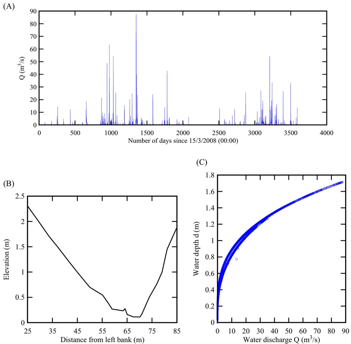
**Fig. 2** Characteristics of the Gara River at Willow Glen north-eastern New South Wales (Data courtesy of NSW DPI Office of Water)—Catchment area: 121 km<sup>2</sup>, site 20635. **a** Hydrograph of the Gara River
