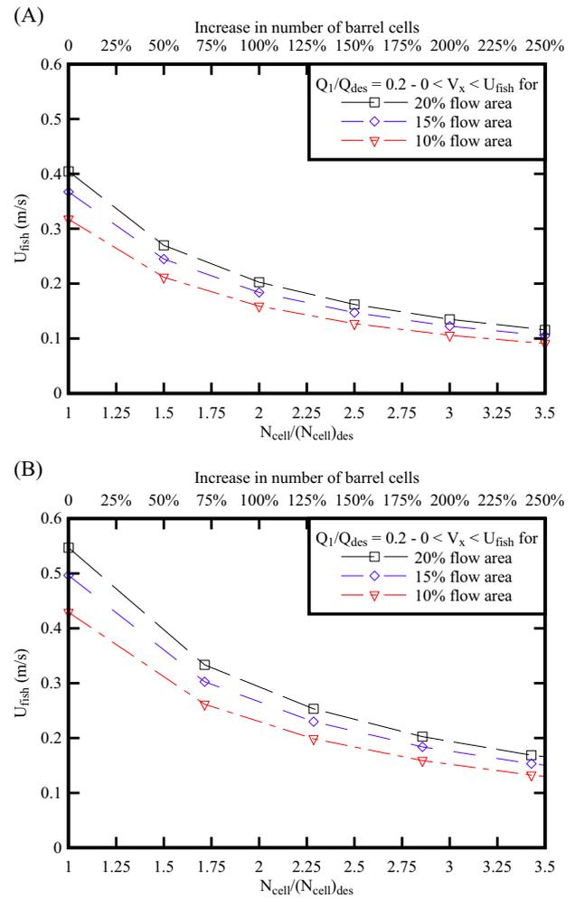
**Fig. 4** Relative increase in number of cells  $N_{cell}/(N_{cell})_{des}$  for fish-friendly multi-cell box culverts as a function of the percentage of LVZ flow area where  $0 < V_x < U_{fish}$  and characteristic fish swimming speed  $U_{fish}$ , for a threshold discharge  $Q_1/Q_{des} = 0.20$ . **a** Culvert 1, **b** Culvert 2
