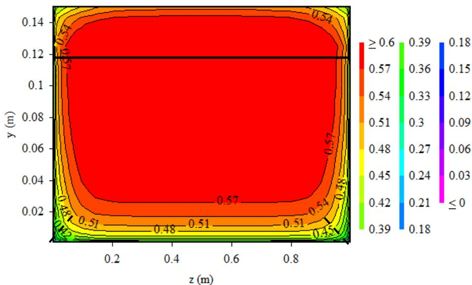
Fig. A-4 - Longitudinal velocity contour of a single cell in a six-cell structure of case 2 (Culvert 2) at 10% of design flow ( $0.1 \times Q_{des} = 0.48 \text{ m}^3/\text{s}$ ); results near the downstream end of the culvert barrel (2 m upstream from the barrel exit); free-surface denoted by solid black line; diagonal length of low velocity zone denoted by black dashed line
