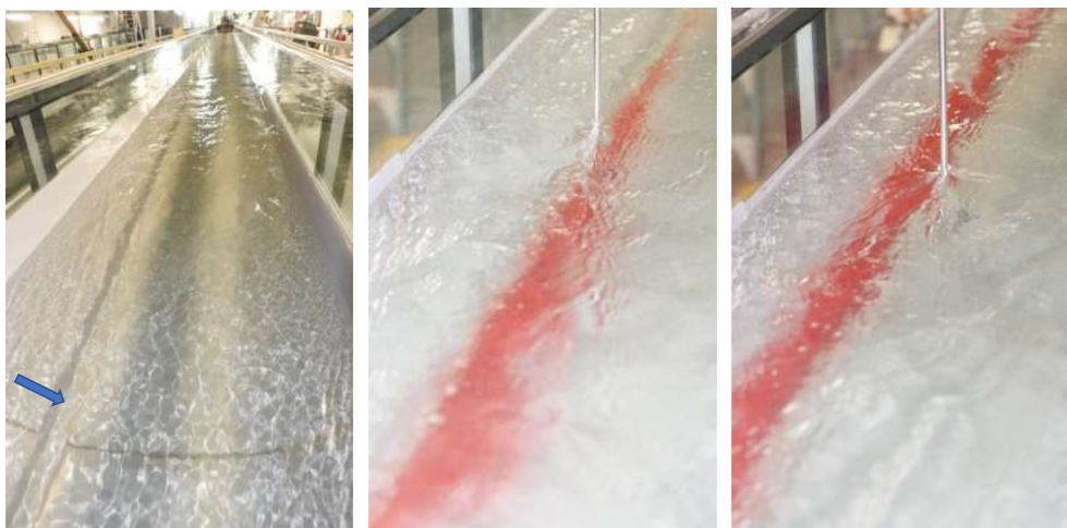
FIGURE 3 Full-scale pipe culvert barrel channel with 0.060 \text{ m} \times 0.020 \text{ m} rail installed at \theta = 30^\circ . Left: Looking upstream for Q = 0.065 \text{ m}^3/\text{s} , with the longitudinal rail seen on the left of the photograph (Arrow). Middle: Dye plume advected along the lower (left) side of the rail for Q = 0.075 \text{ m}^3/\text{s} . Right: Dye plume advected along the upper (right) side of the rail for Q = 0.075 \text{ m}^3/\text{s} . The dye was injected at x = 2.0 \text{ m} and the photograph were taken at x = 7.15 \text{ m} looking upstream [Color figure can be viewed at wileyonlinelibrary.com ]
