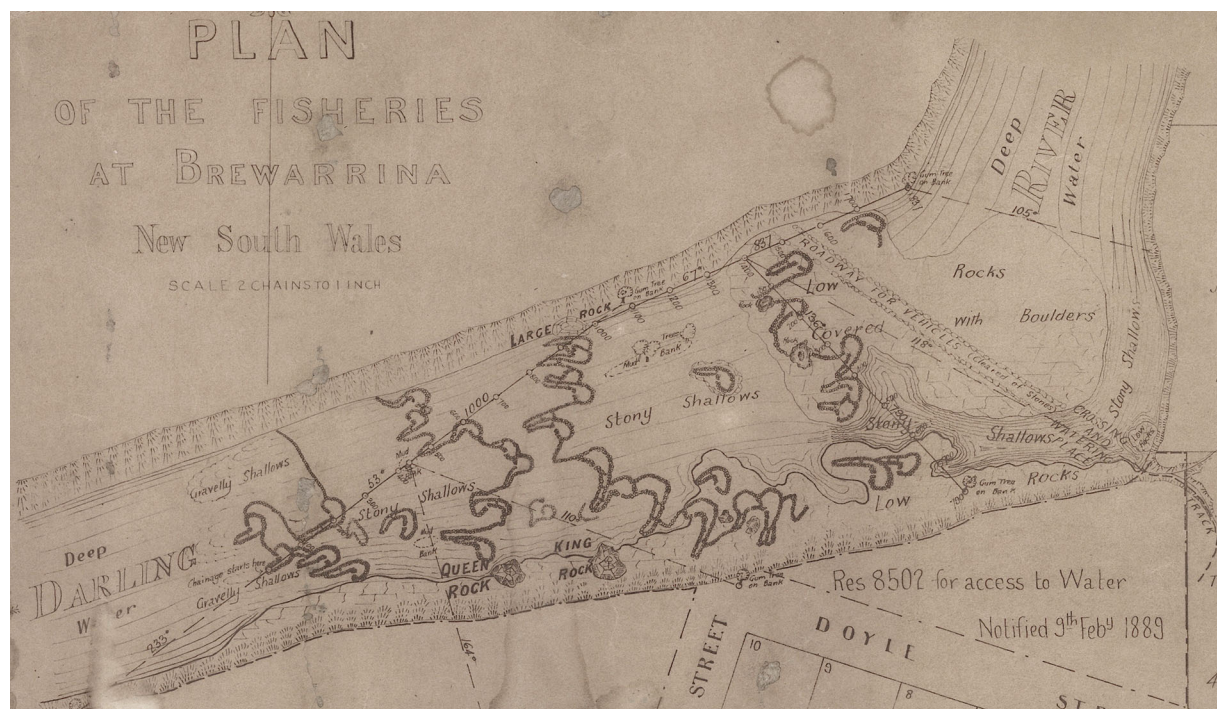
FIGURE 2. Plan of Brewarrina fish traps drawn in 1906 by A. W. Mullen, surveyor to the Western Lands Board (in North, 1916 Plate XXVII). Water flows from right to left.
