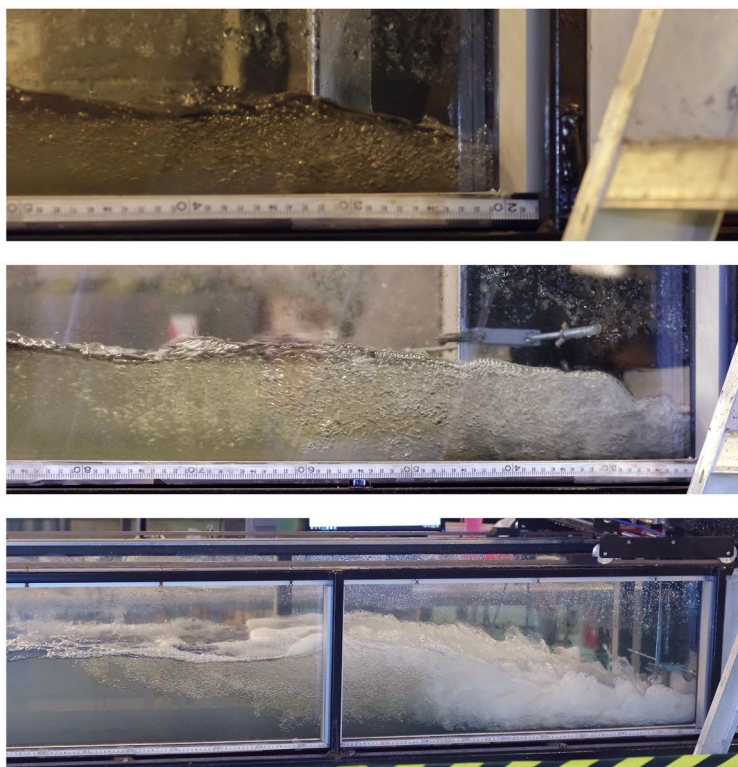
Fig. 2 Photographic observations. a Vertical supported plunging jet channel: (Left) V_1 = 2.46 m/s; (Right) V_1 = 4.5 m/s, b horizontal hydraulic jump channel: (Top) V_1 = 1.79 m/s; (Middle) V_1 = 2.46 m/s (Bottom) V_1 = 4.5 m/s—Flow direction from right to left
