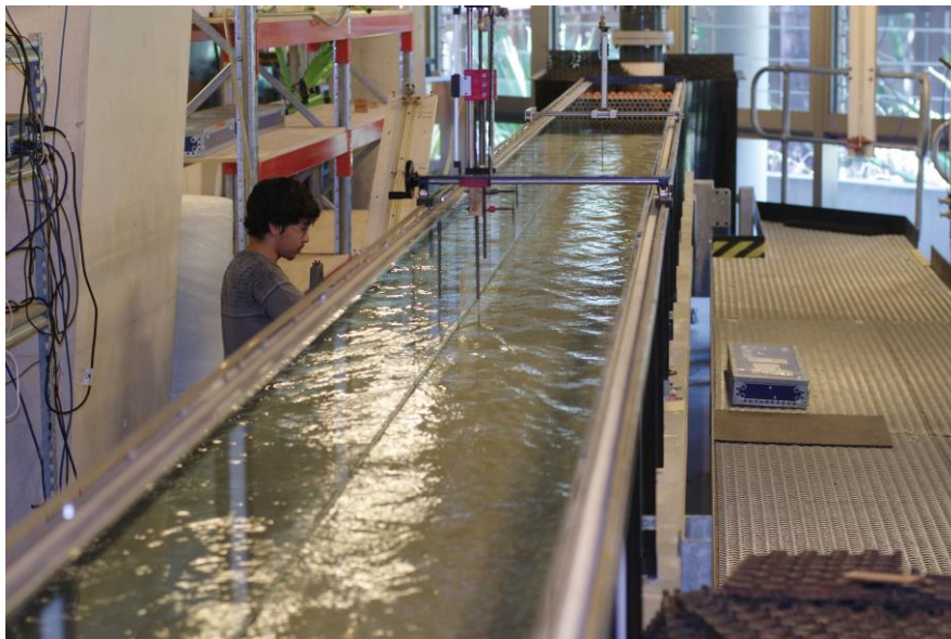
Figure 4. Free-surface flow looking upstream for Q = 0.00556 \text{ m}^3/\text{s} . Note the roving Preston tube (RPT) measurements beneath the sidewall rib (also Fig. 2c) and the intake structure in the background. Flow direction from background to foreground.
