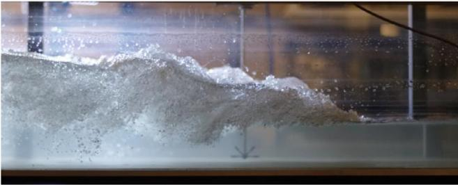
(B) Laboratory experiment - Flow conditions:  $Q = 0.099 \text{ m}^3/\text{s}$ ,  $Fr = 2.1$ ,  $S_0 = 0.0077$ , bore propagation from left to right (shutter speed: 1/1,000 s)
