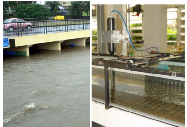
Figure 1. Physical modelling of culvert hydrodynamics. Left: prototype operation in Brisbane on 20 May 2009; Right: laboratory channel with rough bed and sidewall configuration
