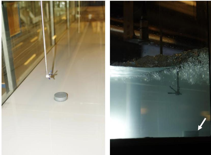
(B, Left) Roughness element in the dry channel looking downstream - (C, Right) Roughness element (white arrow) beneath an advancing bore - Flow conditions:  $Q = 0.061$  m<sup>3</sup>/s,  $d_1 = 155$  mm at  $x = 5.9$  m,  $Fr_1 = 1.39$
