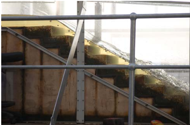
Figure 2. Skimming flow down the gation stepped weir model - Flow conditions: q = 0.147 \text{ m}^2/\text{s} , d_c/h = 1.3 , Re = 5.8 \times 10^5 .
