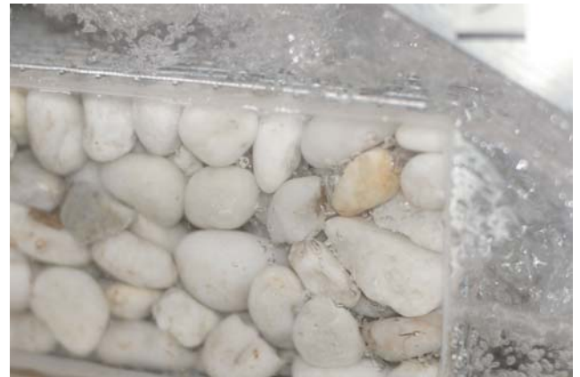
Figure 3. Cavity and gation aeration in skimming flow - Overflow direction from top left to bottom right - Note bubble motion on the gation (shutter speed: 1/180s, flash).
