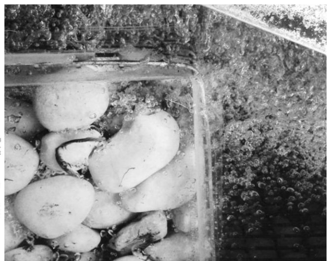
(B) Bubbly motion inside gabions – flow from left to right, 1/5,435 s
