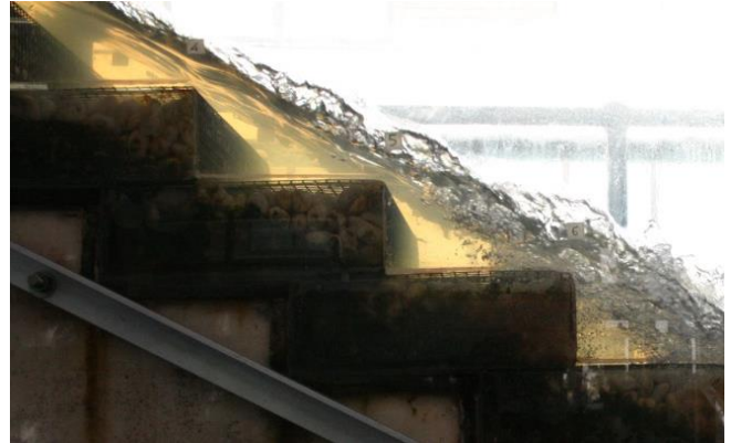
(B) Skimming flow, d_0/h = 1.2 , Re = 5.2 \times 10^5
