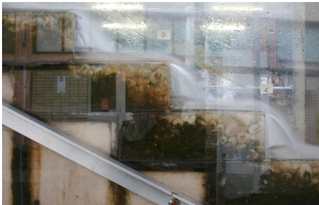
(A) Nappe flow, d_0/h = 0.27 , Re = 5.6 \times 10^4
