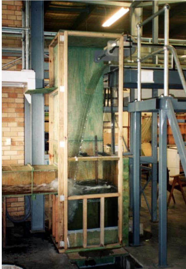
Figure 2. Dropshat in operation with Q=12 L/s
