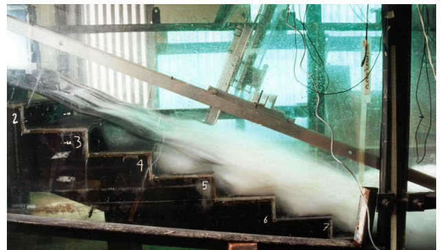
Fig. 2 – Turbulent flows down a stepped chute. Top : Transition flow ( q_w = 0.108 \text{ m}^2/\text{s} , h = 0.1 \text{ m} , l = 0.35 \text{ m} ); detail of air-water flow structures with probe in foreground, view from upstream . Bottom : Skimming flow ( q_w = 0.114 \text{ m}^2/\text{s} , h = 0.1 \text{ m} , l = 0.25 \text{ m} ); flow from the left to the right
