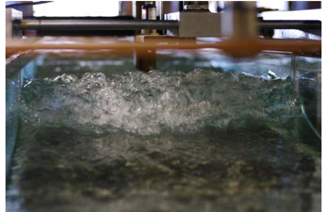
(A) Looking downstream at the advancing breaking bore roller: Q = 0.050 m 3 /s, d_0 = 0.120 m, Fr = 1.58 , fixed gravel bed, shutter: 1/60 s.
