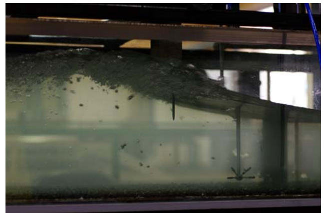
(B) Bore propagation from left to right: Q = 0.050 m 3 /s, d_0 = 0.125 m, Fr = 1.5 , fixed gravel bed, shutter: 1/100 s. Note the underwater bubble "trail" behind the bore roller (Left) and the ADV head on the right.
