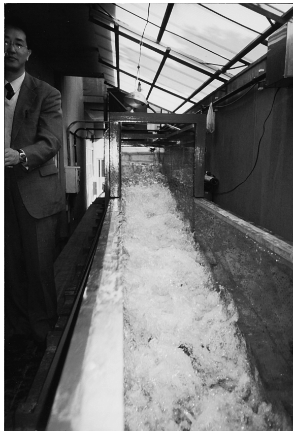
Fig. 3. Photograph of chute flow in operation. Stepped chute flow, Q = 0.033 \text{ m}^3/\text{s} (2,850 \text{m}^3/\text{day} ), \tan\theta = 20\% , h = 0.1 \text{ m} , b = 0.4 \text{ m} . View from downstream (flow from top to bottom).
