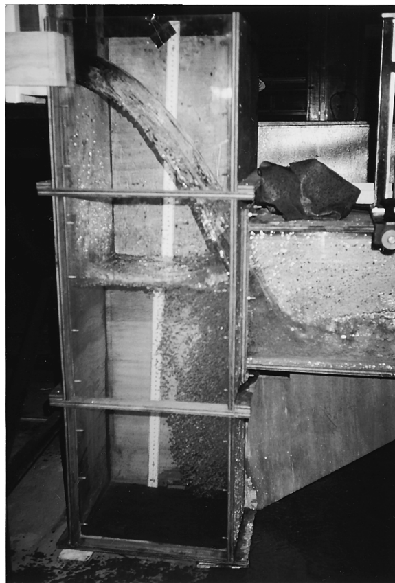
Fig. 17. Photograph of the Recret dropshaft model in operation. Regime R2, Q = 0.00975 \text{ m}^3/\text{s} , h/L = 1.68 , D/L = 0.83 , d_c/L = 0.259 . Side view, flow from left to right. High-speed photograph ( \sim 50 \mu\text{s} ).
