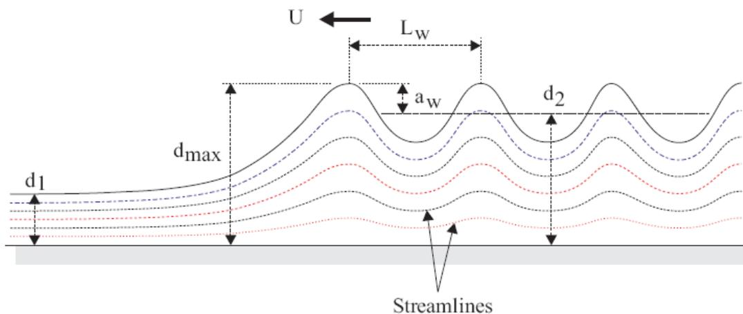
**Fig. 2** - Definition sketch of an undular tidal bore
