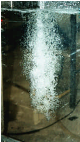
Fig. 2 - Sketch of air entrainment at vertical circular plunging jet
