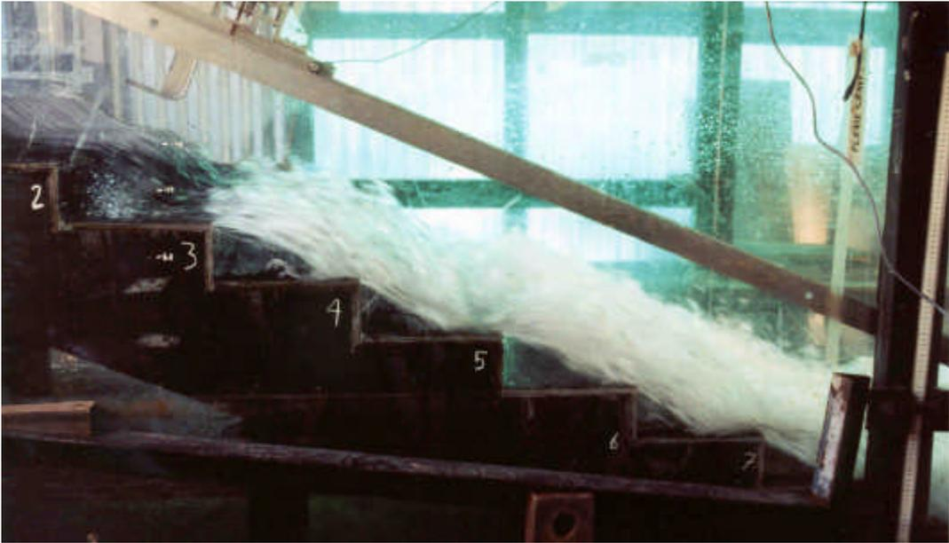
Fig. 3-2 - Flow patterns next to the inception point of free-surface aeration
