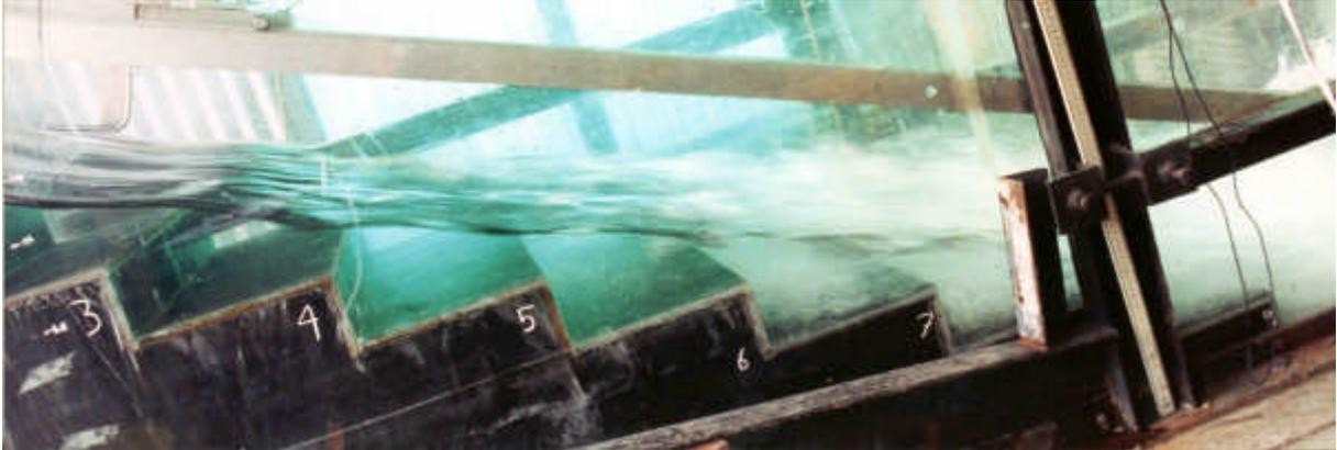
(B) Transition flow ( $d_c/h = 0.7$ ) - Photograph with high shutter speed (1/2,000 sec.)
