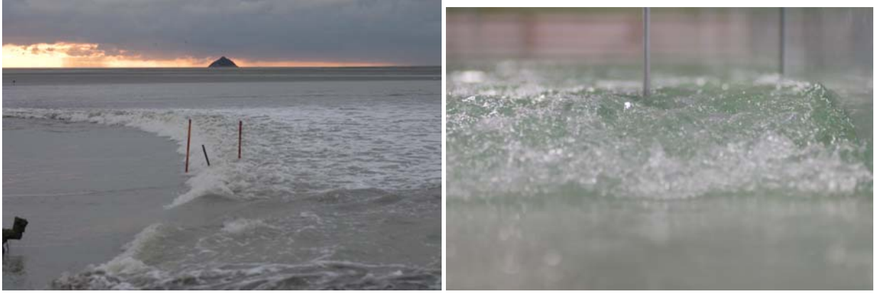
FIG. 1 (Left) - Tidal bore of the Sélune River on 24 September 2010 evening, with bore propagation from right to left - Fr_1 = 2.35 , d_1 = 0.375 m, B_1 = 35 m, U = 2 m/s
