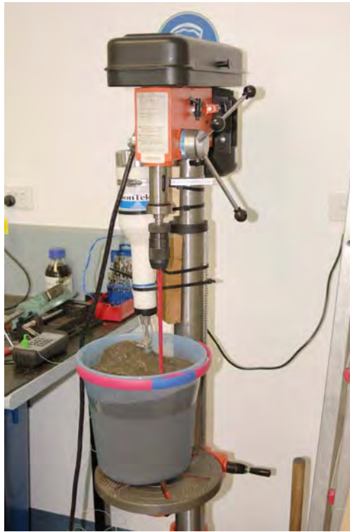
(A) Test for SSC = 70.5 \text{ kg/m}^3 - The ADV system is in the background with the water mixers slightly to the right
