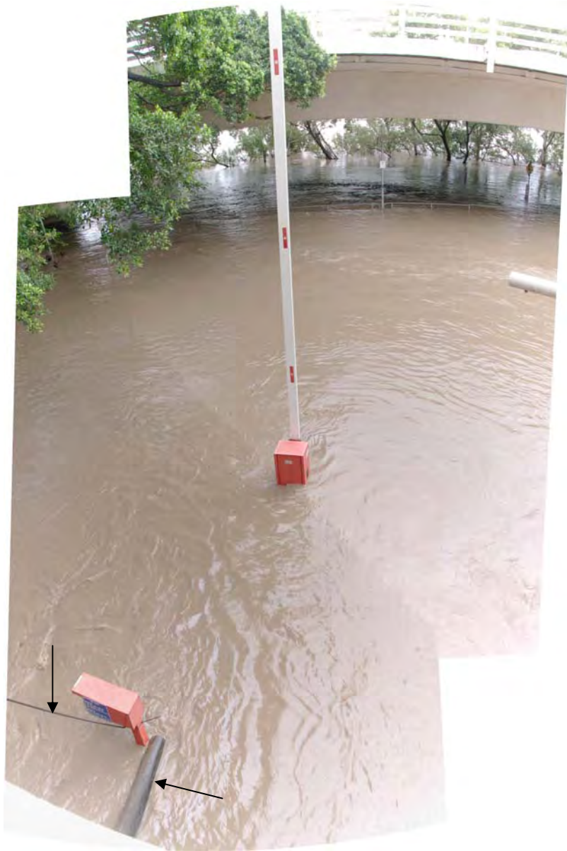
(B) Panoramic shot made from several photographs - Note the timber log jammed in the boom gate pylon and the stretched ADV cable (see arrows)
