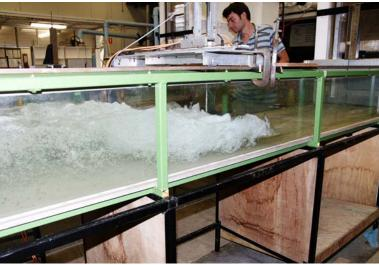
Large air-water projections above the hydraulic jump looking downstream towards the jump toe and air-water projections immediately behind the impingement point. Flow direction from foreground to background. Note the air-water structures projected more than  $5 \times d_1$  above the upstream water surface.  $d_1 = 0.0395$  m,  $Fr_1 = 5.1$ ,  $Re = 1.2 \times 10^5$ . Shutter: 1/180 s at f/2.5, ISO 100.
