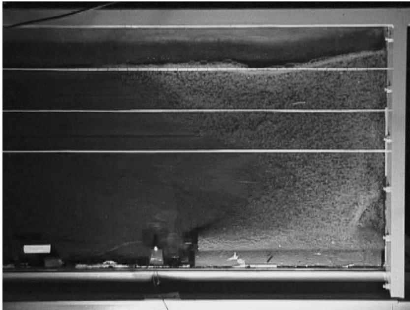
Fig. 6. Free-surface levels in the air injection experiment (Series 2). (A) Photograph taken at  $t=3$  s ( $t_{inj}=20$  s,  $d_1=0.5$  m); (B) sketch of free-surface flow pattern next to the injection point; (C) dimensionless free-surface elevations  $Y$  (measured above still water level) next to the origin after air bubble injection ( $T_{inj}>8$ ).
