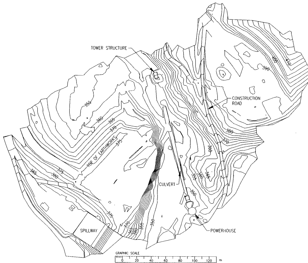
Fig. 4. Topographic contour plan of breached Opuha Dam immediately following dam failure
