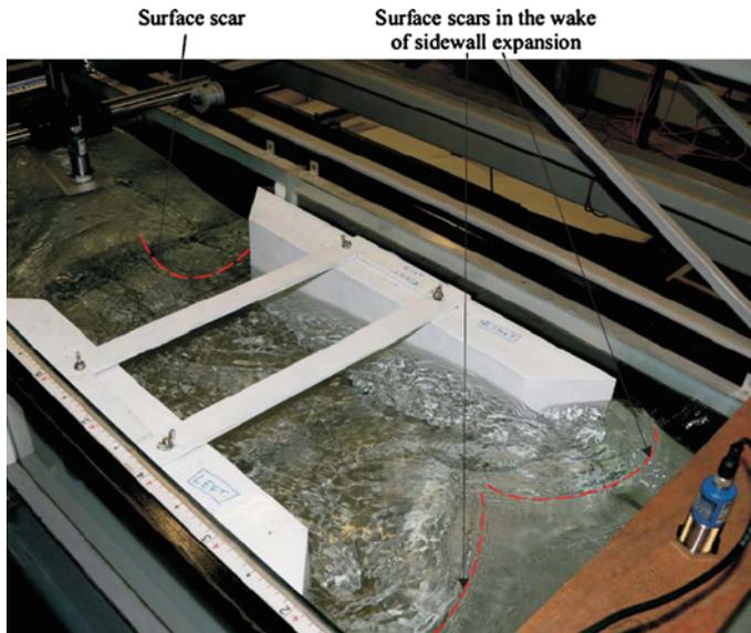
**Fig. 6** First wave crest of the undular bore ( $Fr = 1.15$ ) exiting the channel constriction—note the complicated turbulent pattern upstream of the channel constriction (right) as well as the surface scars in the throat and in the diverging constriction—bore propagation from *top left* to *bottom right*, Shutter speed: 1/80 s—run 090318\_00,  $Q = 0.0232 \text{ m}^3/\text{s}$ ,  $d_0 = 0.1552 \text{ mm}$  (at  $x = 3.6 \text{ m}$ ),  $Fr = 1.15$ ,  $U = 1.10 \text{ m/s}$
