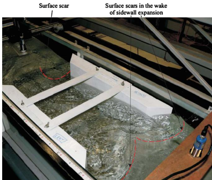
**Fig. 6** First wave crest of the undular bore ( $\text{Fr} = 1.15$ ) exiting the channel constriction—note the complicated turbulent pattern upstream of the channel constriction (right) as well as the surface scars in the throat and in the diverging constriction—bore propagation from top left to bottom right, Shutter speed: 1/80 s—run 090318\_00,  $Q = 0.0232 \text{ m}^3/\text{s}$ ,  $d_0 = 0.1552 \text{ mm}$  (at  $x = 3.6 \text{ m}$ ),  $\text{Fr} = 1.15$ ,  $U = 1.10 \text{ m/s}$
