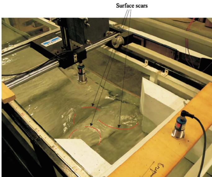
**Fig. 5** Undular tidal bore, looking at the first wave crest entering the constriction—note the free-surface turbulence and scars next to the throat convergent—shutter speed: 1/50 s—run 090415\_61,  $Q = 0.0089 \text{ m}^3/\text{s}$ ,  $d_0 = 0.0845 \text{ mm}$  (at  $x = 3.6 \text{ m}$ ),  $\text{Fr} = 1.16$ ,  $U = 0.85 \text{ m/s}$
