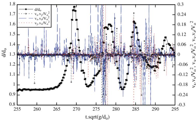
**Fig. 14** Dimensionless water depth and tangential stresses in an undular bore in a rectangular channel—downstream of constriction:  $x = 5 \text{ m}$ ,  $z/d_0 = 0.312$ , run 090424\_901c,  $d_0 = 0.1147 \text{ m}$  at  $x = 3.6 \text{ m}$ ,  $V_0 = 0.3313 \text{ m/s}$ ,  $U = 1.05 \text{ m/s}$ ,  $Fr = 1.16$
