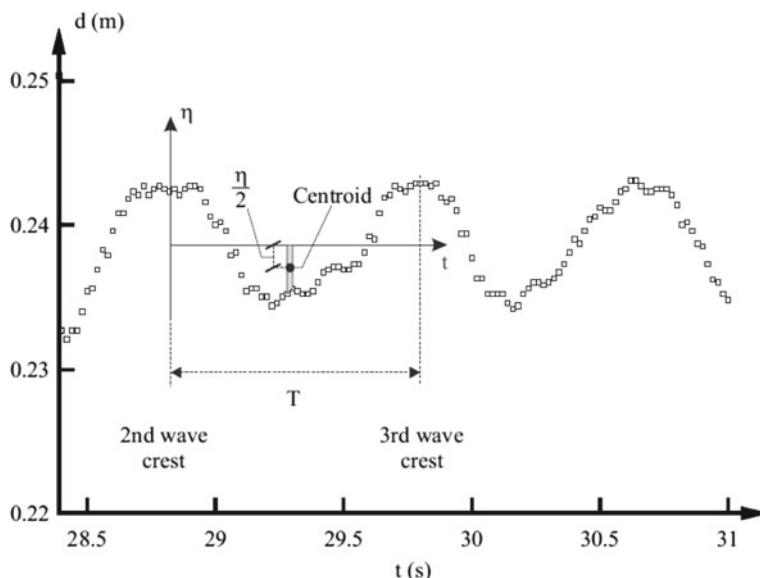
**Fig. 8** Potential energy integration along the second wave length—experimental data: Run 090417\_63,  $x = 5$  m,  $Q = 0.0190 \text{ m}^3/\text{s}$ ,  $d_0 = 0.212$  m at  $x = 3.6$  m,  $\text{Fr} = 1.04$ ,  $U = 1.32 \text{ m/s}$
