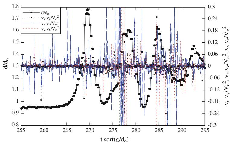
**Fig. 14** Dimensionless water depth and tangential stresses in an undular bore in a rectangular channel—downstream of constriction:  $x = 5$  m,  $z/d_0 = 0.312$ , run 090424\_901c,  $d_0 = 0.1147$  m at  $x = 3.6$  m,  $V_0 = 0.3313$  m/s,  $U = 1.05$  m/s,  $Fr = 1.16$
