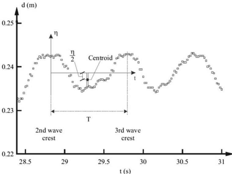
**Fig. 8** Potential energy integration along the second wave length—experimental data: Run 090417\_63,  $x = 5$  m,  $Q = 0.0190$  m<sup>3</sup>/s,  $d_0 = 0.212$  m at  $x = 3.6$  m,  $Fr = 1.04$ ,  $U = 1.32$  m/s
