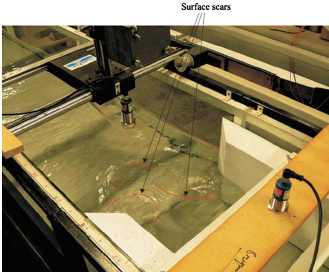
**Fig. 5** Undular tidal bore, looking at the first wave crest entering the constriction—note the free-surface turbulence and scars next to the throat convergent—shutter speed: 1/50 s—run 090415\_61,  $Q = 0.0089 \text{ m}^3/\text{s}$ ,  $d_0 = 0.0845 \text{ mm}$  (at  $x = 3.6 \text{ m}$ ),  $Fr = 1.16$ ,  $U = 0.85 \text{ m/s}$
