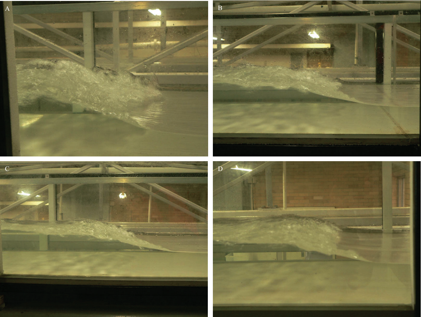
Figure 3. Photographs of a decelerating surge front propagating upstream against a steep slope: S_o = 0.00943 , Q = 0.0354 \text{ m}^3 \text{ s}^{-1} , d_o = 0.0538 \text{ m} (Series 2). Initial flow from right to left, surge propagation from right to left. (A) t = 12.3 \text{ s} , x_s = 8 \text{ m} ( U = 0.18 \text{ m s}^{-1} , breaking); (B) t = 31.5 \text{ s} , x_s = 5 \text{ m} ( U = 0.10 \text{ m s}^{-1} , breaking); (C) t = 48.2 \text{ s} , x_s = 3 \text{ m} ( U = 0.075 \text{ m s}^{-1} , breaking); (D) t = 67.5 \text{ s} , x_s = 1 \text{ m} ( U = 0.05 \text{ m s}^{-1} , breaking). This figure is available in colour online at wileyonlinelibrary.com
