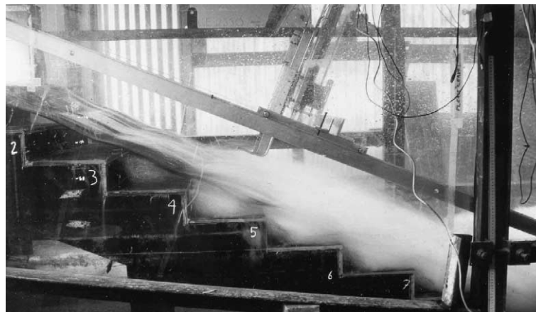
Fig. 3. Experimental flow conditions: skimming flow ( q_w = 0.114 \text{ m}^2/\text{s} , h = 0.1 \text{ m} , l = 0.25 \text{ m} ); flow from the left to the right; note the inception of free-surface aeration downstream of the step edge 4, and the probe travelling mechanism.
